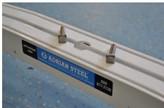
Crossbar with T-Slot and square-head bolts.
